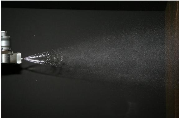
An increase in fluid pressure increases the velocity of the impinging fluid jets and increases the fluid fan width. If the fan is too wide for the flow rate required the emission rate will increase and the user should change to a tip with larger fluid passages and / or a smaller impingement angle.
